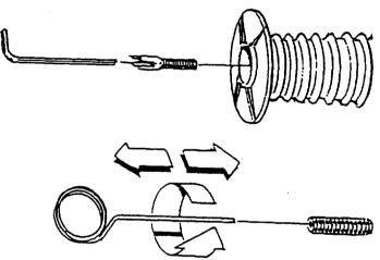
Insert wire into nozzle and turn back and forth to clear obstruction.
